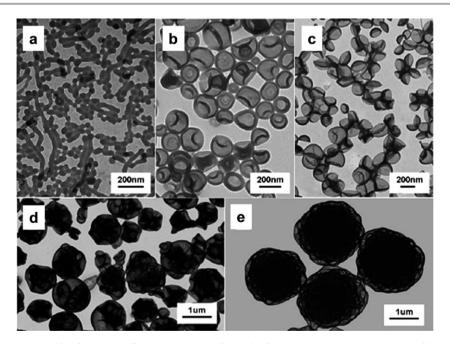
Fig. 6 TEM images of PAA-b-PSt assemblies formed at different molar ratios after 20 h of polymerization. St/PAA-TTC = 250 (a), 500 (b), 750 (c), 1000 (d), and 1250 (e).19
