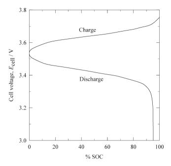
**Fig. 6** Cell voltage *vs.* normalized capacity characteristics of a lithium-ferricyanide flow battery during charge-discharge. <sup>92</sup> (SOC: state of charge.)
