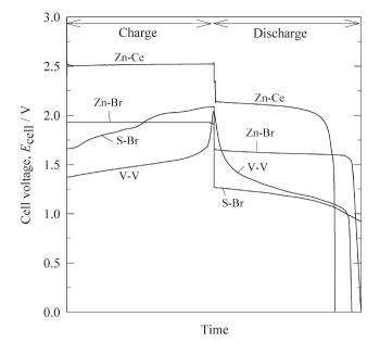
Fig. 12 Cell voltage vs. time response during charge/discharge for all-vanadium (30 mA cm<sup>-2</sup> for 2 h),<sup>44</sup> zinc-bromine (15 mA cm<sup>-2</sup> for 10 h),<sup>164</sup> bromine-polysulfide (40 mA cm<sup>-2</sup> for 30 mins)<sup>213</sup> and the undivided zinccerium (20 mA cm<sup>-2</sup> for 30 mins)<sup>17</sup> redox flow batteries.
