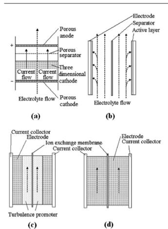
Fig. 8 Schematics of (a) a flow-through, (b) a flow-by electrode; (c) two-dimensional and (d) three-dimensional electrode configurations for a redox flow battery  $^{98,201}$
