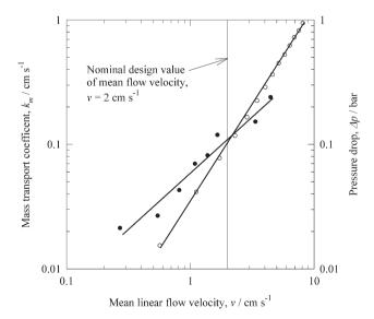
**Fig. 11** Log-plots of (a) ● mass transport coefficient and (b) ○ pressure drop *vs.* mean linear electrolyte velocity for the bromine compartment of the polysulfide-bromine redox flow battery. Electrolyte: 1 mol dm<sup>-3</sup> NaBr in 0.5 mol dm<sup>-3</sup> Na<sub>2</sub>SO<sub>4</sub> at pH 2.<sup>277</sup>
