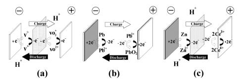
Fig. 4 Types of redox flow battery, according to the nature of energy storage. Energy is stored (a) in the electrolytes, (b) in the active material within the electrodes and (c) hybrid (in both electrode and electrolyte phases).
