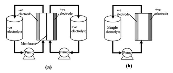
Fig. 1 The principle of (a) a divided and (b) an undivided (membraneless) redox flow battery.
