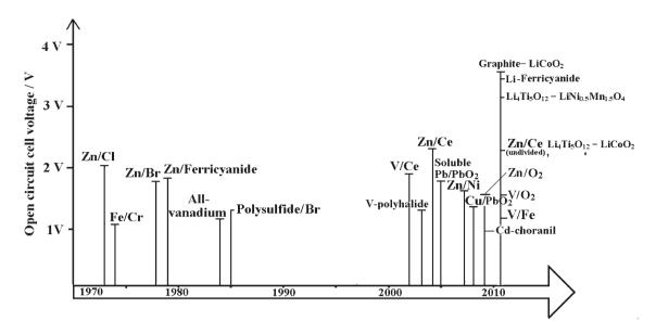
Fig. 3 The timeline of the development of redox flow batteries over the past 40 years.
