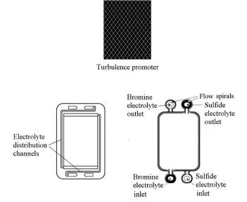
Fig. 10 Schematics of turbulence promoter, flow frame and spiral-shaped flow paths. 276,277
