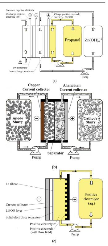
Fig. 5 Examples showing configurations of three types of flow batteries: (a) zinc-oxygen bifunctional, <sup>188</sup> (b) lithium flowable electrode <sup>91</sup> and (c) lithium-aqueous ferricyanide flow batteries.<sup>93</sup>
