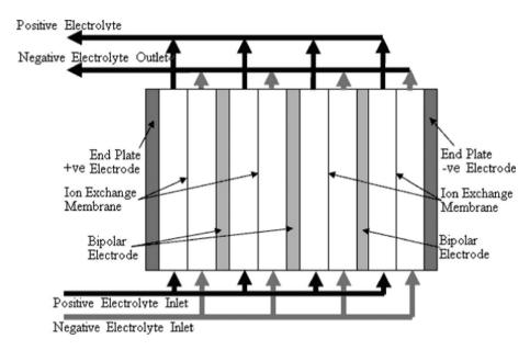
Fig. 2 A stack design for a four cell stack with bipolar connection of electrodes.<sup>8</sup>
