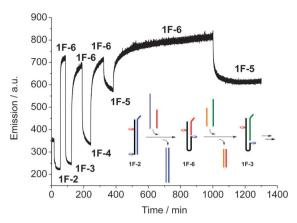
**Fig. 3** Real-time monitoring of the switching between the five different switching states, recording acceptor emission ( $\lambda_{\rm ex}=495~{\rm nm}$ ,  $\lambda_{\rm em}=583~{\rm nm}$ ), and schematic drawing of the first steps. The final switches between **1F.6** and **1F.5** show the reversibility and stability of the system.
