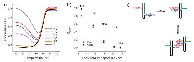
Fig. 2 (a) Fluorescence melting curves of the DNA switch by monitoring FAM emission ( $\lambda_{ex} = 495$  nm,  $\lambda_{em} = 510$  nm); (b) calculated vs. experimental FRET of the modified system in the FAM and TAMRA system 1F; (c) putative intra- and intermolecular stacking of the porphyrins in the DNA beacon systems.
