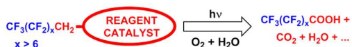
Scheme 2 Proposed formation of perfluoroalkyl carboxylate from fragmentation of long-chain fluororous compound in environment.
