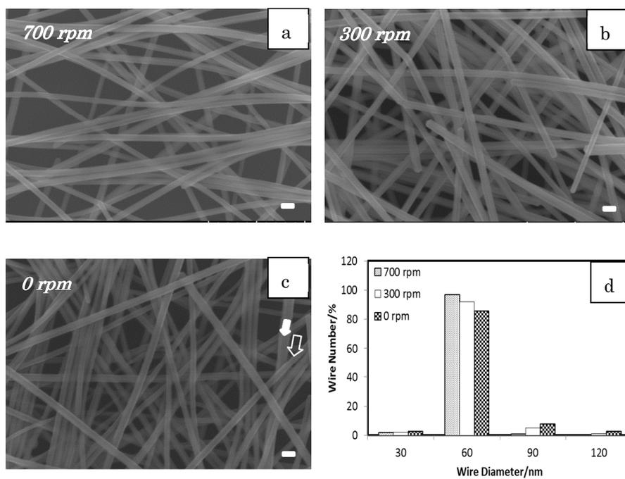
Fig.3. The SEM images of AgNWs prepared at 130 °C with stirring speeds (a, b and c with the scale bar of 100 nm), and related diameter distribution (d).
