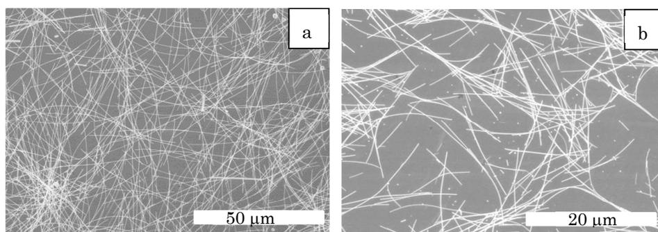
Fig.2. The SEM images of AgNWs prepared at 110 (a) and 180 °C (b) without agitation.
