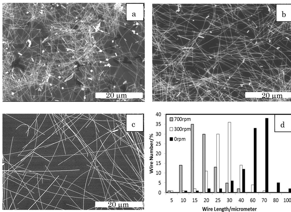
Fig.1. The SEM images of AgNWs prepared at 130 °C with stirring speeds of (a) 700, (b) 300 and (c) 0 rpm (those inserted photos have a scale bar of 30μm), and the length distribution of AgNWs with different stirring speeds (d).
