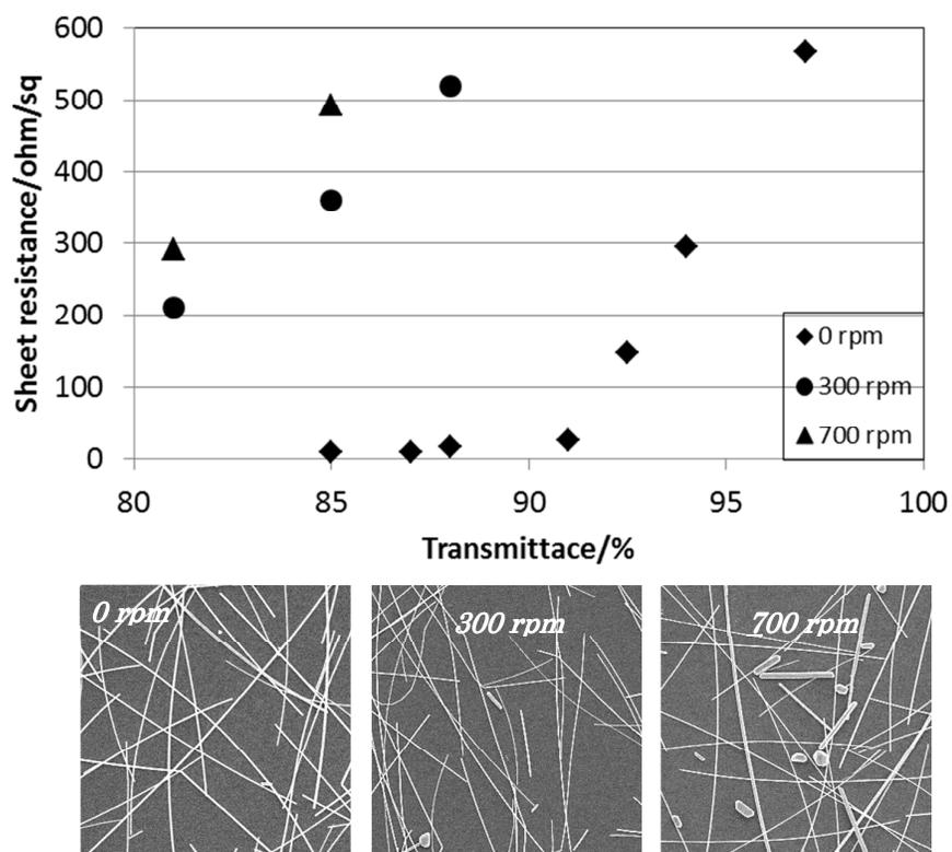
Fig.4 The relationship between sheet resistance and transmittance of AgNWs film on glass substrate and film SEM images with transmittance of 85 % at 550 nm (the side length is 15  $\mu\text{m}$ ).
