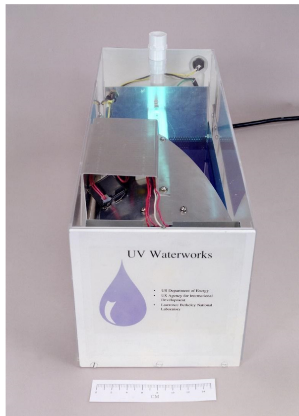
Fig. 13 UV waterworks, built with a glass cover for exhibits and displays to explain how the technology works.
