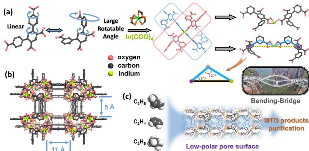
Fig. 1 Structural description of ZJNU-401: (a) from the "bending-bridge" design of the ligand to the assembly with mononuclear In<sup>3+</sup> to form the 4-c node; (b) 1D pore channel of ZJNU-401; (c) low-polarity pore surface for effective MTO product purification.
