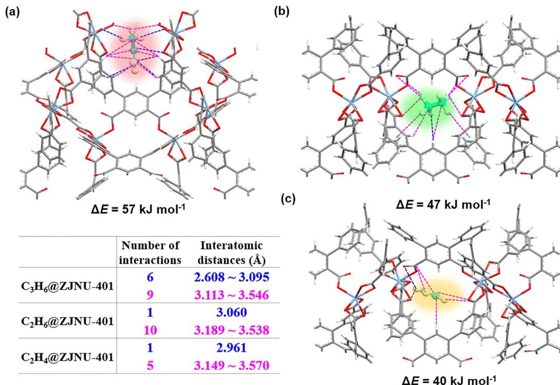
Fig. 3 Calculation of the optimized adsorption sites for (a) C<sub>3</sub>H<sub>6</sub> and (b) C<sub>2</sub>H<sub>6</sub> and (c) C<sub>2</sub>H<sub>4</sub> within ZJNU-401, and comparison of the host–guest interactions among them.
