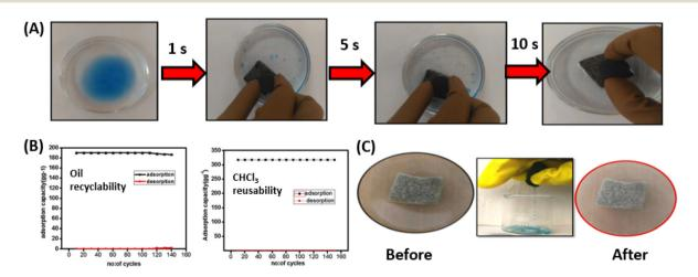
Fig. 10 (A) Oil removal by magnetically driven GPUF over time; (B) adsorption capacity of GPUF in cycles of adsorption and desorption of diesel oil and chloroform; (C) digital images of GPUF before and after reusability studies using diesel oil (reproduced from ref. 115. Copyright 2020 Elsevier Inc.).
