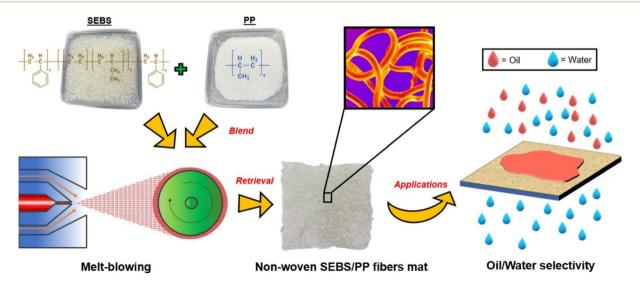
Fig. 16 Schematic diagram of SEBS/PP fibers mat fabricated through melt-blowing. Reproduced from ref. 191, Copyright 2023 Elsevier Inc.
