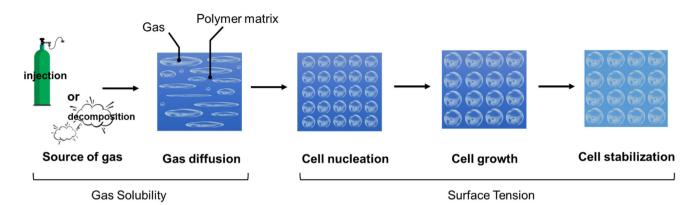
Fig. 5 Cell-formation procedure of polymeric foam.
