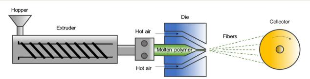
Fig. 13 Melt-blowing process from the extruder.
