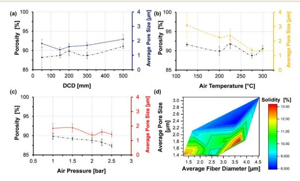
Fig. 15 Porosity and pore size of PP melt-blown fibers as a function of (a) die-to-collector distance, (b) air temperature, (c) air pressure; (d) 2D contour plot of fiber solidity and pore size as a function of fiber diameter. (Reproduced from ref. 174. Copyright 2021 John Wiley & Sons, Inc.)
