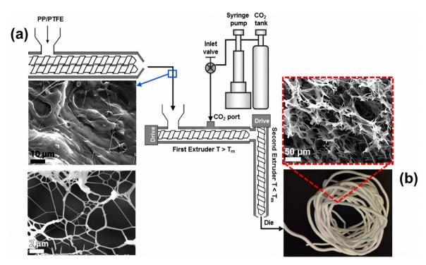
Fig. 7 Extrusion foaming of PP/PTFE fibrillar blends: (a) PP-homopolymer blended with PTFE in a twin-screw extruder; (b) images of an open-cell foam filament produced via extrusion. (Reproduced from ref. 91, Copyright 2014 American Chemical Society.)
