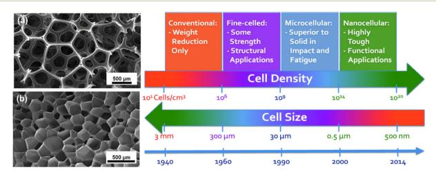
Fig. 4 (a) Open-cell 59 and (b) closed-cell<sup>60</sup> structures of polymeric foams; (c) cell sizes and cell density of the developed foams over time.<sup>66</sup> (Reproduced from ref. 59, 60 and 66. Copyright 2004 and 2005 Elsevier Inc.)
