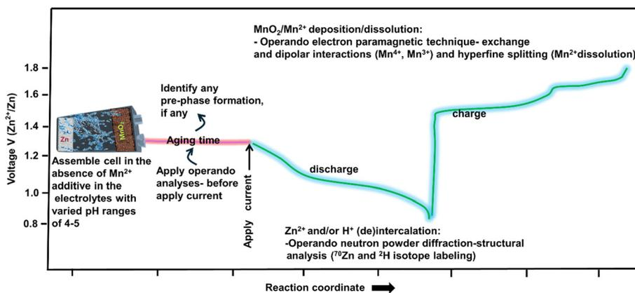
Fig. 3 Plausible forecast road map to distinguish  $\text{Zn}^{2+}$  vs.  $\text{H}^+$  intercalation from  $\text{MnO}_2/\text{Mn}^{2+}$  electrodeposition–dissolution in layered  $\text{MnO}_2$  through isotope labeling, operando neutron and electron paramagnetic resonance analyses.
