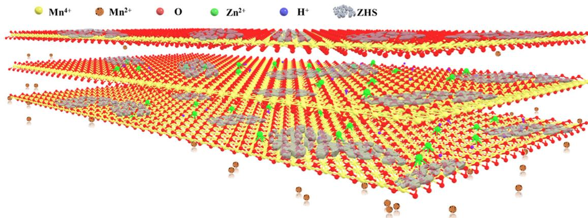
**Fig. 1** With conflicting electrochemical reaction mechanisms in aqueous Zn–MnO<sub>2</sub> batteries, possible proposed storage mechanisms include Mn electrodedissolution–deposition, H<sup>+</sup> and/or Zn<sup>2+</sup> intercalation–deintercalation and ZHS (Zn<sub>4</sub>(OH)<sub>6</sub>SO<sub>4</sub>·nH<sub>2</sub>O) deposition–dissolution are depicted in δ-MnO<sub>2</sub>, a layered phase, from a pool of available MnO<sub>2</sub> polymorphs.
