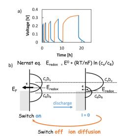
Fig. 6 Voltage behaviour of n-Si/Ge/copper ionic electrolyte/FTO at 80 °C, 100 nA discharge and recovery (a); 45 conceptual diagram of Nernst's equation (b); blue: discharge (switch on), orange: recovery (switch off).  $E_{\rm F}$ : Fermi level.  $E_{\rm O}$ : standard redox potential.  $c_{\rm o}$ ,  $c_{\rm R}$ : concentration of oxidized and reduced elements. Do, DR: density of states of oxidized and reduced ions (Copyright © 2019 Royal Society of Chemistry)
