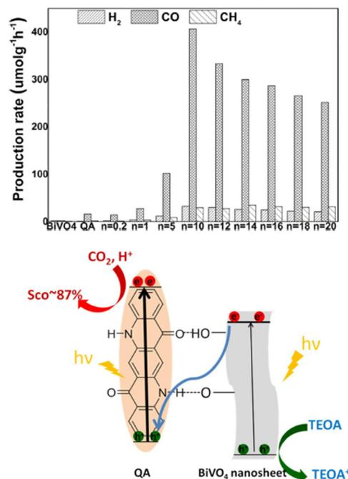
Fig. 8 Top panel: Production rates from CO<sub>2</sub> photoreduction (average over 10 h) on BiVO<sub>4</sub>, QA, and QA/*n*BiVO<sub>4</sub> for 10 h. *n* is the mass ratio between BiVO<sub>4</sub> and QA, impacting the photocatalytic performance. Bottom panel: Schematic representation of photochemical CO<sub>2</sub> reduction on QA/BiVO<sub>4</sub> composites. Reproduced from ref. 50 with permission from Wiley Inc., copyright 2020.
