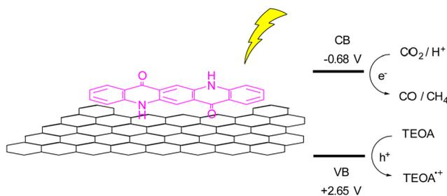
Fig. 7 Reduction of CO<sub>2</sub> over QA/rGO photocatalyst, and schematic representation of CO<sub>2</sub> reduction to CO and CH<sub>4</sub>, coupled with oxidation of triethanolamine (TEOA); the potential of the conduction and valence bands (CB and VB, respectively) are reported versus the reversible hydrogen electrode.<sup>49</sup>
