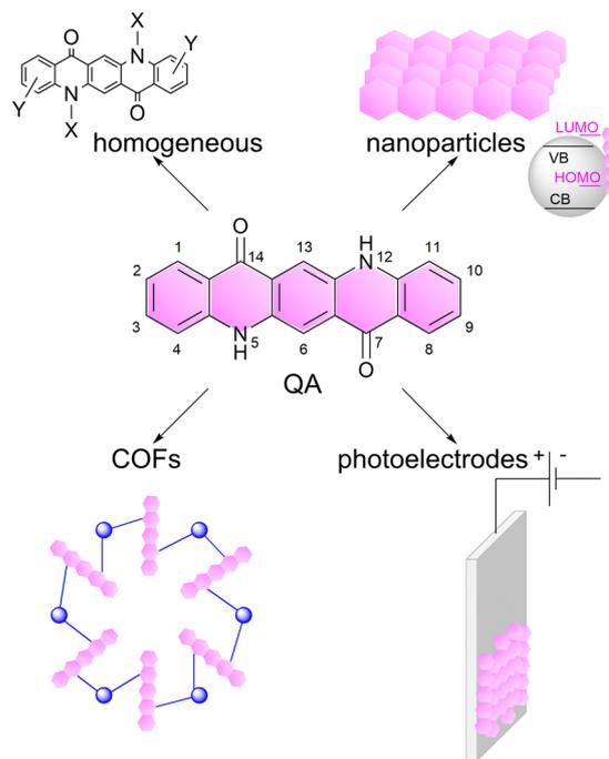
**Scheme 1** Representation of the linear *trans*-isomer of quinacridone (QA), and of its versatility for application in photo- and photo-electrocatalysis, which is the subject of this perspective article. The numeration of the atoms in QA scaffold is also reported.<sup>25</sup>
