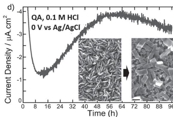
**Fig. 12** (a) and (b) Epindolidione (EPI) and QA photocathodes for photoelectrochemical synthesis of H<sub>2</sub>O<sub>2</sub> upon reduction of oxygen. Panel (c) represents the operating mechanism and the energy levels involved. Panel (d) shows the morphological evolution of QA films along the photoelectrocatalysis by scanning electron microscopy. Reproduced from ref. 39 with permission from Wiley Inc., copyright 2016.
