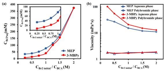
Fig. 3 Ex situ characterization of electrolytes containing initial (pre-partition) bromine concentration ranging from 0.25 M to 2 M, as well as 2 M ZnBr<sub>2</sub>, and 0.5 MEP or 3-MBPy. (a) Measured bromine concentration in the aqueous phase at equilibrium, versus initial bromine concentration. (b) Measured viscosity of each phase versus initial bromine concentration
