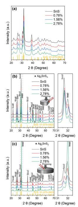
Fig. 1 Powder X-ray diffraction (PXRD) patterns collected from SnS and Ag-doped SnS powders (a) and the surfaces of sintered samples parallel to (b) and perpendicular to (c) the pressing direction.
