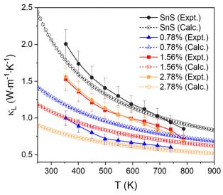
Fig. 7 Comparison of the measured in-plane lattice thermal conductivity  $\kappa_{\rm L}$  and the calculated  $\kappa_{\rm L}$  of pristine and Ag-doped SnS.
