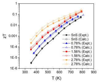
Fig. 8 Thermoelectric figure of merit zT of pristine and Ag-doped SnS ceramics. For each set of samples two sets of data are given: one obtained using the measured lattice thermal conductivity  $\kappa_1$  ("expt", solid lines/solid symbols) and one using the calculated  $\kappa_1$  ("calc.", dashed lines/open symbols)
