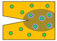
Cavitation and shear banding
