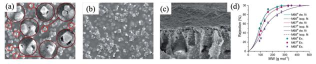
Fig. 25 SEM images of (a) UiO-66-NH $_2$  MMM (top view), (b) UiO-66-PNIPAM MMM (top view), and (c) cross-sectional UiO-66-PNIPAM MMM. (d) Rejection performance of the experimental results (dots) and fitted MWCO curves for MMM with PNIPAM-grafted UiO-66 (M66 $^{P}$ ), UiO-67 (M67 $^{P}$ ), and UiO-68 (M68 $^{P}$ ). Copyright 2021 Royal Society of Chemistry.
