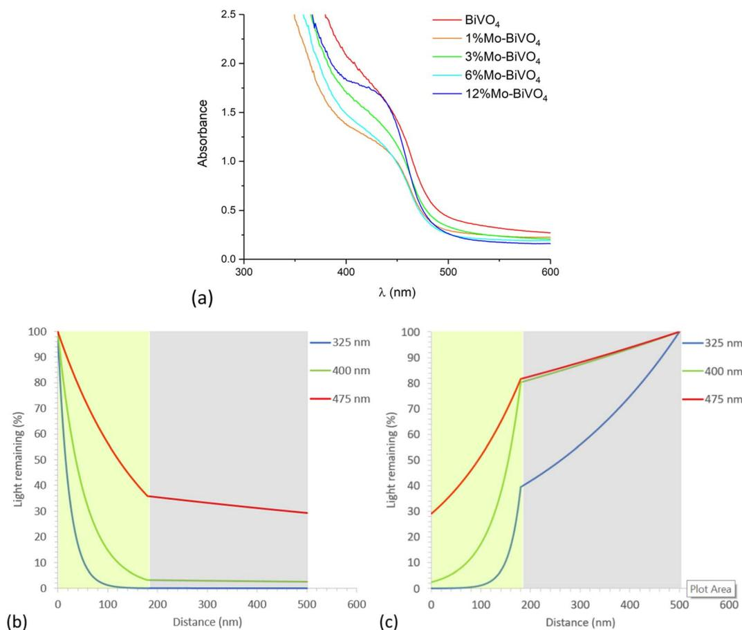
Fig. 5 (a) UV-visible absorption spectra of  $\text{BiVO}_4$  and all Mo-doped  $\text{BiVO}_4$  samples and light remaining (%) with distance travelled in 6% Mo- $\text{BiVO}_4$  for (b) front irradiation and (c) back irradiation (shaded green and grey areas represent  $\text{BiVO}_4$  [180 nm thick] and FTO [320 nm thick] layers respectively).
