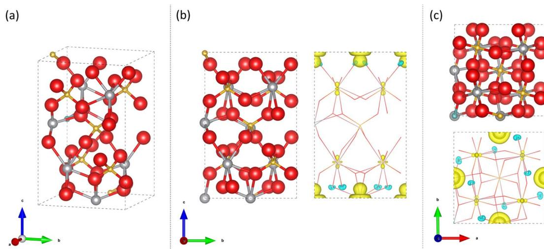
Fig. 10 Calculated structure for 12.5 at% Mo doping of a V site in tetragonal scheelite  $\text{BiVO}_4$  for a single unit cell showing atomic positions and spin density [Bi = silver, V = gold, O = red, Mo = light blue; ionic radii proportions scaled down for visibility]. (a) Angled view, (b)  $a$ -axis view and (c)  $c$ -axis view.
