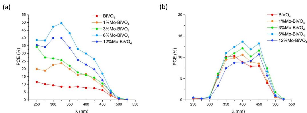
Fig. 7 Incident photon to current efficiency (IPCE) curves for BiVO<sub>4</sub> and all Mo-doped BiVO<sub>4</sub> samples measured with (a) front irradiation and (b) back irradiation. Samples were measured in 0.1 M phosphate buffer (pH = 7) at 1.23 V<sub>RHE</sub>.
