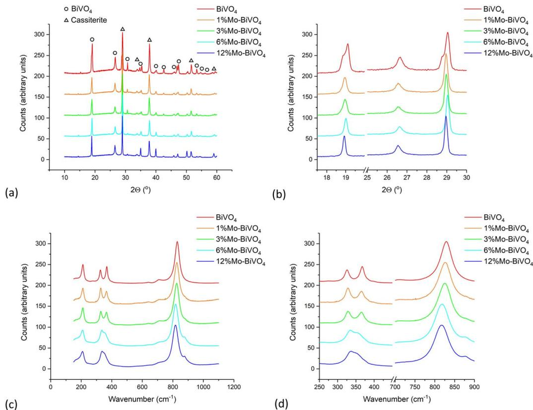
Fig. 2 (a) XRD patterns, (b) close-up view of select peaks in XRD patterns, (c) Raman spectra and (d) close-up view of select peaks in Raman patterns of  $\text{BiVO}_4$  and all Mo-doped  $\text{BiVO}_4$  samples.
