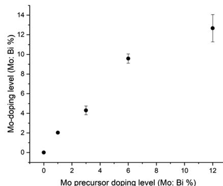
**Fig. 3** A plot of the relationship between Mo precursor dopant level (Mo : V %) vs. the Mo doping level determined by XPS analysis. All values are the average of 3 unique sample locations; with the error bars representing one standard deviation.
