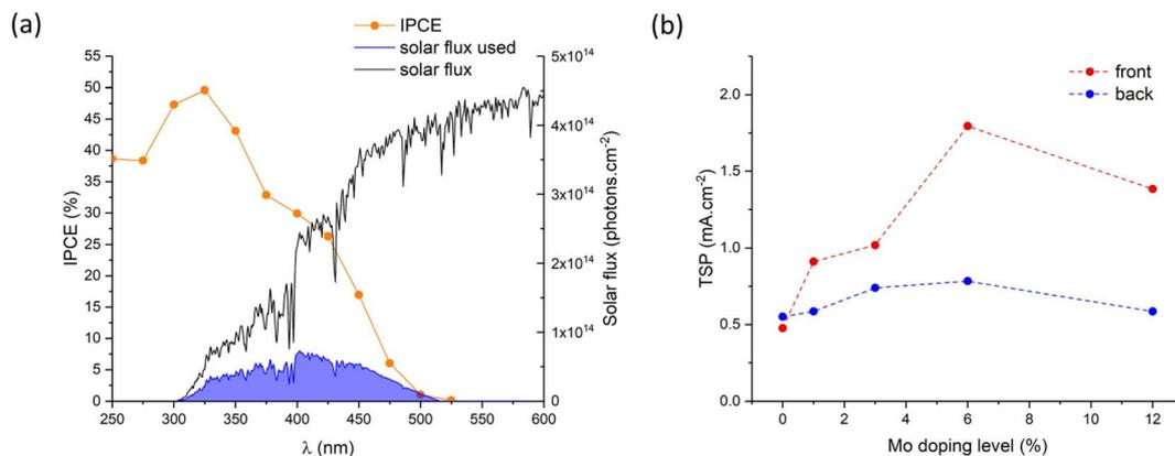
Fig. 8 (a) Calculation of the theoretical solar photocurrent (TSP) for 6% Mo-BiVO<sub>4</sub> under front irradiation at 1.23 V<sub>RHE</sub> and (b) a summary of the TSP photocurrents at 1.23 V<sub>RHE</sub> for front and back irradiation as a function of Mo precursor doping level (%) of BiVO<sub>4</sub> and all Mo-doped BiVO<sub>4</sub> samples.
