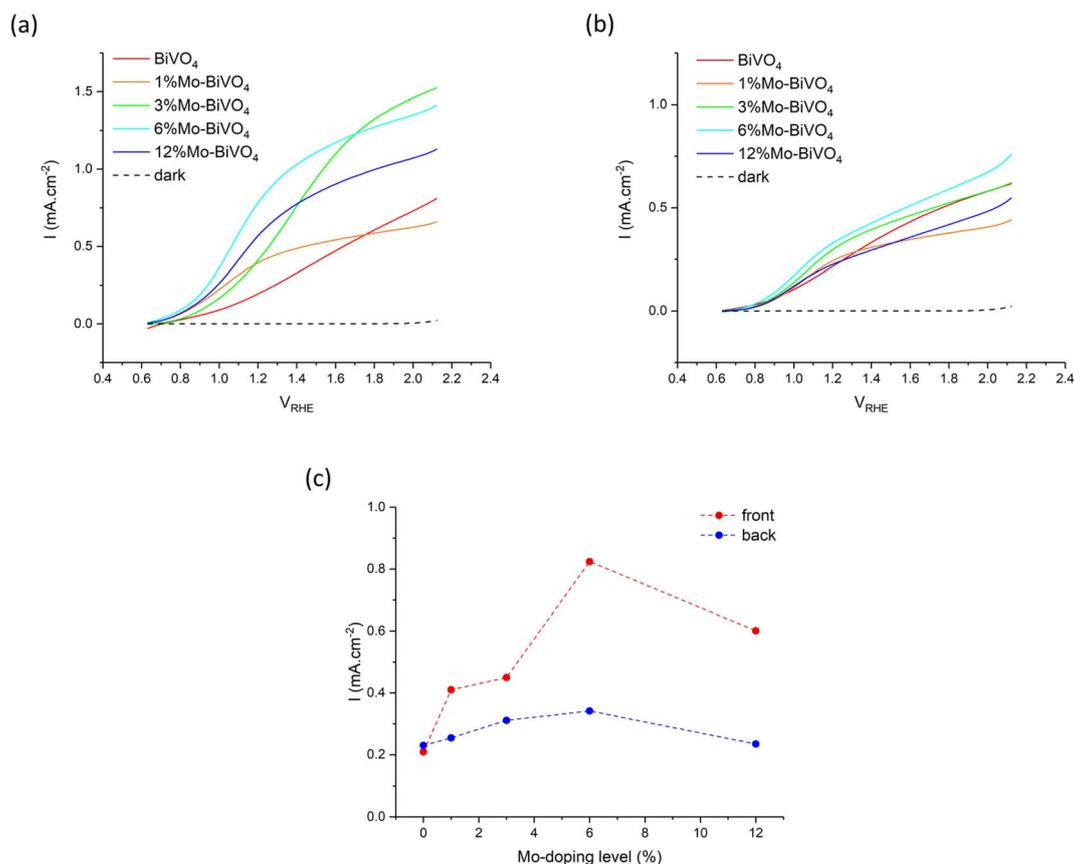
Fig. 6 Current voltage ( $JV$ ) curves for  $\text{BiVO}_4$  and all Mo-doped  $\text{BiVO}_4$  samples measured with (a) front irradiation and (b) back irradiation. (c) The photocurrent densities observed at  $1.23 V_{\text{RHE}}$  for both front and back irradiation as a function of Mo precursor doping level (%) of  $\text{BiVO}_4$  and all Mo-doped  $\text{BiVO}_4$  samples. Samples were measured in 0.1 M phosphate buffer (pH = 7) using 400 nm light ( $\sim 8.5 \text{ mW cm}^{-2}$ ).
