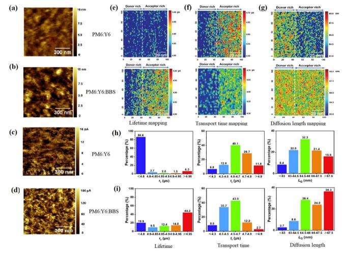
Fig. 4 AFM-topography of (a) PM6:Y6, and (b) PM6:Y6: BBS. c-AFM-conductivity of (c) PM6:Y6 and (d) PM6:Y6: BBS. (e) Carrier lifetime ' $\tau_r$ ', (f) carrier transport time ' $\tau_t$ ', (g) carrier diffusion length  $L_D$ . (h and i) Statistical distribution of  $\tau_r$ ,  $\tau_t$ , and  $L_D$  for PM6:Y6 and PM6:Y6: BBS organic films.<sup>60</sup> Reproduced from ref. 60 with permission from John Wiley and Sons, copyright 2022.
