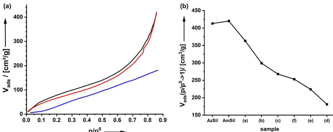
Fig. 3 (a) H<sub>2</sub>O vapor adsorption of AzSil (black), AmSil (red) and Am<sub>0.48</sub>Sp(d)<sub>0.42</sub>Sil (blue). (b) Water uptake at  $p/p^0 = 0.86$  for different organosilica materials.
