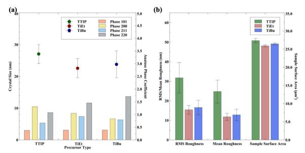
Fig. 6 The effect of the precursor type on (a) average crystal properties and (b) average surface properties ( $R_{\alpha}$  roughness and SSA) seen across the 58 samples produced herein (TTIP = 22 samples; TiEt = 14 samples; TiBu = 22 samples). Error bars represent 80% confidence intervals.
