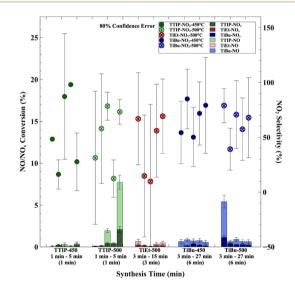
Fig. 4 Photocatalytic  $NO/NO_x$  conversion (bar chart) and  $NO_2$  selectivity (scatter chart) of samples grown with varying synthesis time for a fixed bubbler temperature of 160 °C (green-TTIP, red-TiEt, and blue-TiBu); the range of times specified represents the range of synthesis times studied from left to right in the bar chart, with times in brackets beneath representing the time intervals between each bar.
