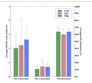
Fig. 7 The effect of the precursor type on average photocatalytic NO<sub>x</sub> activity seen across the 58 samples produced herein (green-TTIP = 22samples; red-TiEt = 14 samples; blue-TiBu = 22 samples). Error bars represent 80% confidence intervals.
