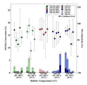
Fig. 5 Photocatalytic  $NO/NO_x$  conversion (bar chart) and  $NO_2$  selectivity (scatter chart) of samples grown at differing bubbler temperatures for a fixed synthesis time of 3 min (green-TTIP, red-TiEt, and blue-TiBu); the range of temperatures specified represent the range of bubbler temperatures studied from left to right in the bar chart, with temperatures in brackets representing the temperature intervals between each bar.
