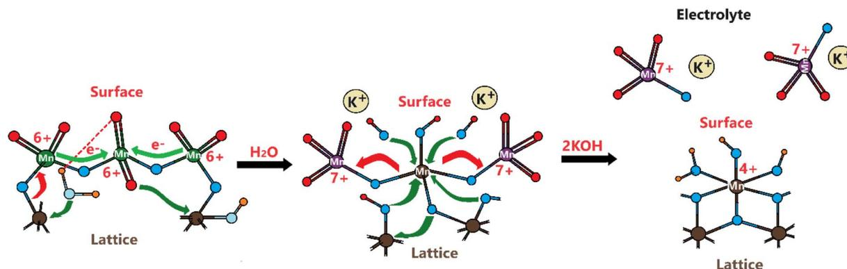
Scheme 1 Electrode degradation mechanism of LiMn<sub>2</sub>O<sub>4</sub> electrodes during the OER.
