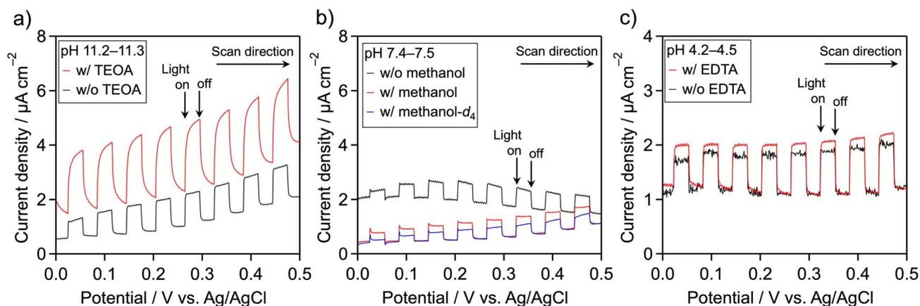
**Fig. 2** Current–potential curves for Pt/meso-PCN/FTO electrodes under an Ar atmosphere and under irradiation with chopped visible light ( $\lambda > 400$  nm), as recorded in aqueous Na<sub>2</sub>SO<sub>4</sub> (0.1 M) containing different additives: (a) TEOA, (b) methanol and (c) EDTA. Scan rate: 10 mV s<sup>-1</sup>. Note: w/ and w/o in the figure indicate with and without, respectively.
