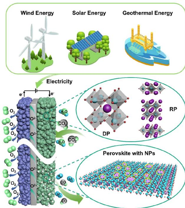
Fig. 1 A typical schematic of an SOEC.
