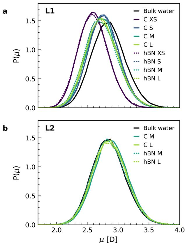
Fig. 4 Dipole moment distribution in the interfacial water layers. Dipole moment distributions obtained from the combined NNP and DFT calculations for the first (a) and second (b) interfacial layers of water on graphene (solid lines) and hBN (dashed lines), as well as bulk water. The distribution is normalized by the isotropic distribution.
