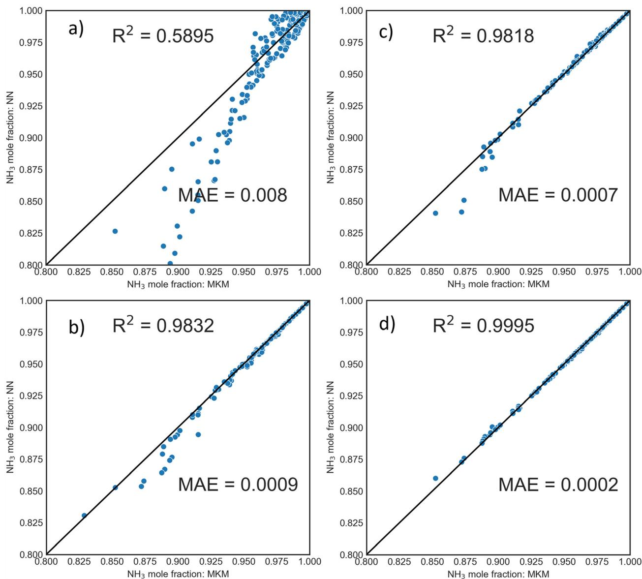
**Fig. 3** Parity plots for PFR exit mole fraction for unseen, randomly chosen operating conditions within the training phase-space using DNNs trained with FF design for a) 100 and c) 400 PFR simulations or LHS sampling for b) 100 and d) 400 PFR simulations.
