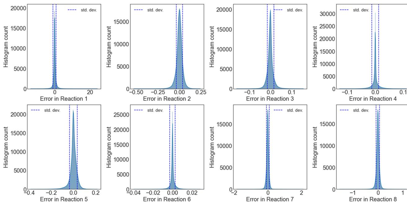
**Fig. 6** Uncertainty quantification of the NN training error for a cumulative 100 independent NNs trained on reaction set B. Errors are deviations of overall rates between NN predictions and MKM calculations. Errors in rates are in 1 s<sup>-1</sup>.
