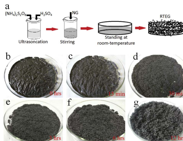
Fig. 9 (a) The schematic diagram of thermally synthesis by the one-step room-temperature method. (b–g) Optical images of the graphite intercalation and morphological evolutions with time from 0 to 12 h. Reprinted with permission from ref. 58
