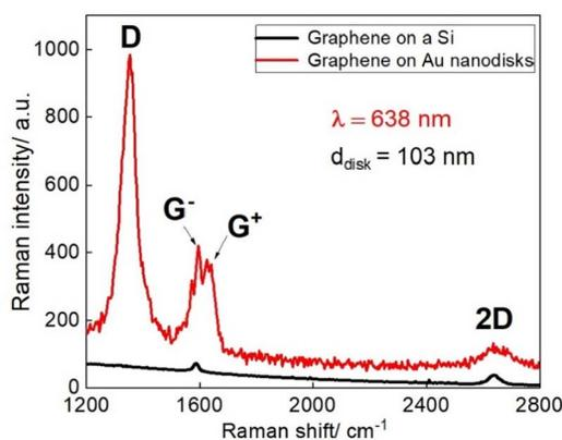
Fig. 2 Typical SERS spectrum of graphene film on a plasmonic substrate (the diameter of gold nanodisks is about 103 nm) (red) and the Raman spectrum of the graphene film measured on a bare Si/SiO<sub>2</sub> substrate (black) at an excitation wavelength of 638 nm.
