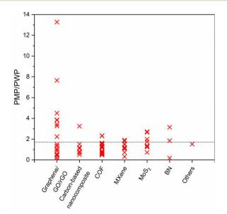
Fig. 10 The ratio of pure methanol permeance (PMP) over pure water permeance (PWP) of free-standing 2D nanolaminate membranes. The dashed line represents the inverse relationship between the viscosity of methanol (0.54 mPa s) and water (0.916 mPa s). Raw data was given in
