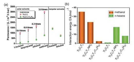
Fig. 6 (a) Comparison of hydrophilic Ti<sub>3</sub>C<sub>2</sub>T<sub>x</sub> and hydrophobic Ti<sub>3</sub>C<sub>2</sub>T<sub>x</sub>-C<sub>12</sub>H<sub>2</sub> membrane permeabilities, and (b) interaction energies between membrane and solvent.<sup>53</sup> This figure has been reproduced from ref. 53 with permission from the Wiley Online Library, Copyright 2019.
