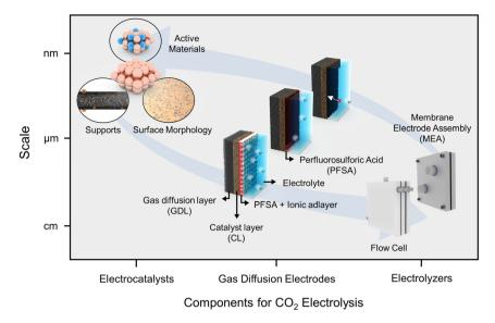
Fig. 1 Strategic insights into the acidic  $CO_2RR$  in terms of scale and components such as electrocatalysts, gas diffusion electrodes, and electrolyzers.
