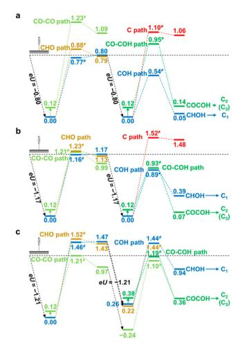
Fig. 5 DFT-based theoretical free energy diagrams of CO<sub>2</sub>RR intermediates according to the electrolyte pH.83 Free energy diagrams under (a) acidic conditions with pH 1, (b) neutral conditions with pH 7, and (c) alkaline conditions with pH 12. Reproduced with permission from ref. 83. Copyright 2016, ACS Publications.
