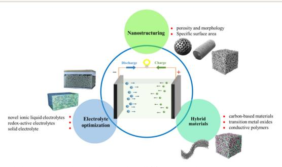
Fig. 13 The strategies for improving the performance of supercapacitors with SiC nanomaterials electrodes
