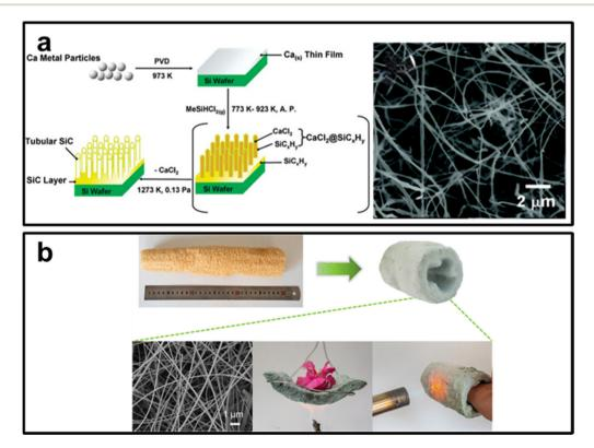
Fig. 8 (a) Large-scale fabrication of single-crystal SiC nanowire sponges using agricultural residue loofah.Reprinted with permission from ref. 127. Copyright 2007 by American Chemical Society; (b) long SiC nanowires grow in the specified direction. Reprinted with permission from ref. 129. Copyright 2023 by American Chemical Society.
