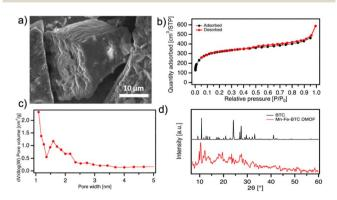
Fig. 2 (a) SEM image of Mn-Fe-BTC DMOF, (b) N<sub>2</sub> isotherm adsorption/desorption isotherm analysis of Mn-Fe-BTC DMOF, (c) pore size distribution of Mn-Fe-BTC DMOF and (d) PXRD spectra of BTC (black) and Mn-Fe-BTC DMOF (red)
