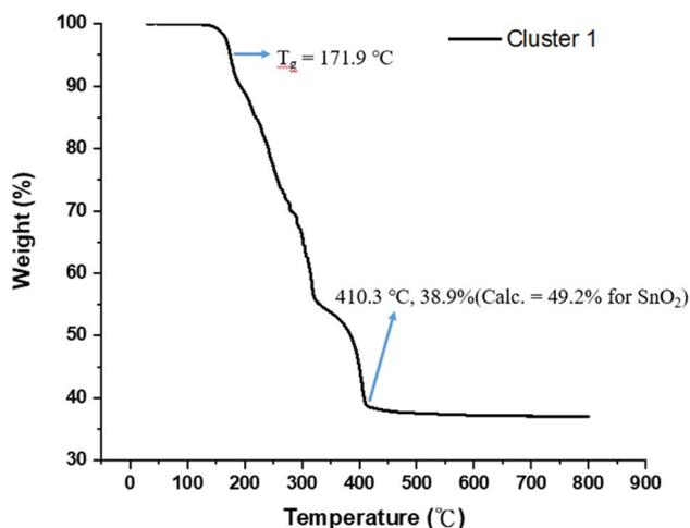
Fig. 1 Thermogravimetric analysis in the 30–800 °C range.
