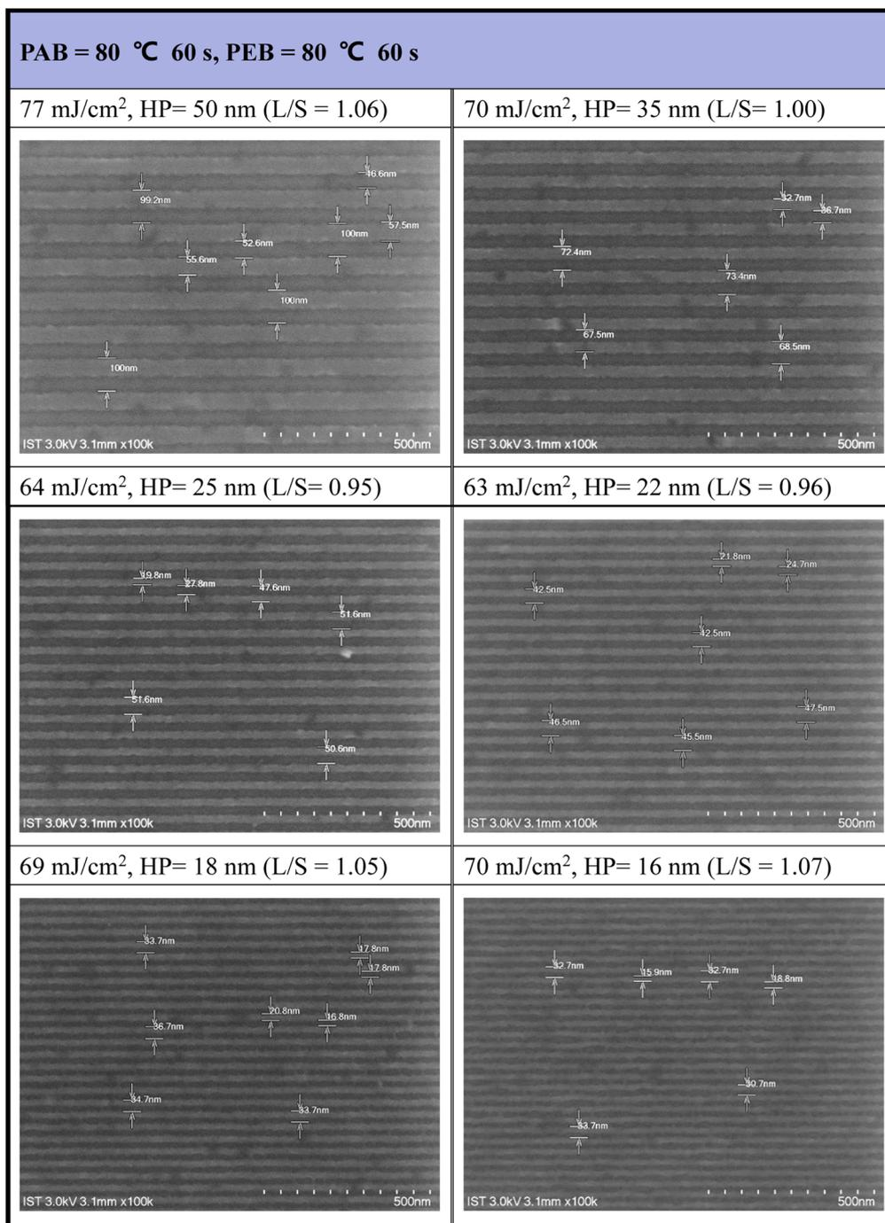
Fig. 7 SEM images of EUV patterns for photoresist (3). Initial thickness 22 nm. PAB (80 °C, 60 s) and PEB (80 °C, 60 s), developer 2-heptanone (60 s).
