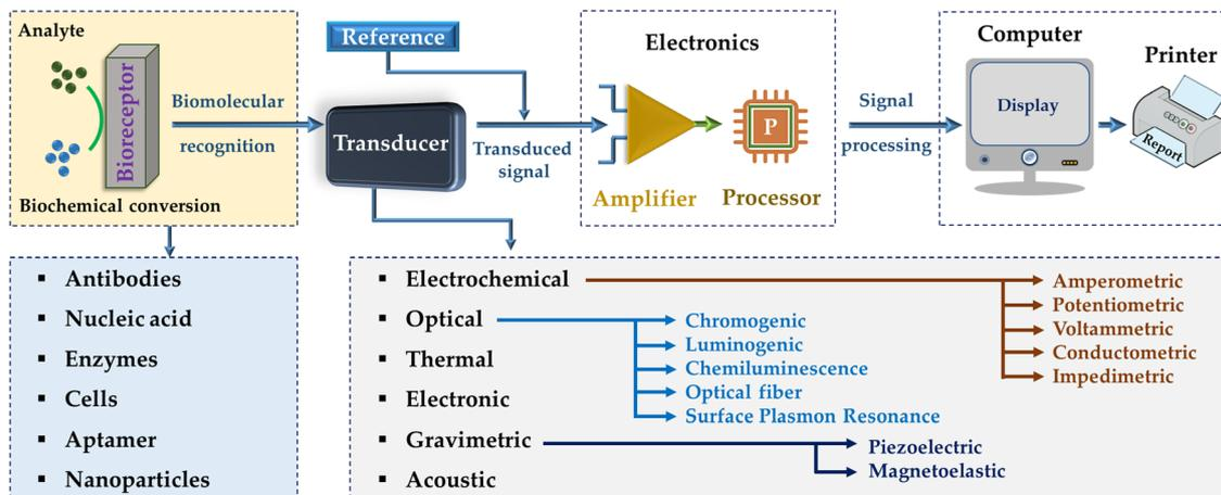
Fig. 1 Schematic illustration of a biosensing device, which is comprised of a bioreceptor, transducer, and amplifier.<sup>42</sup>
