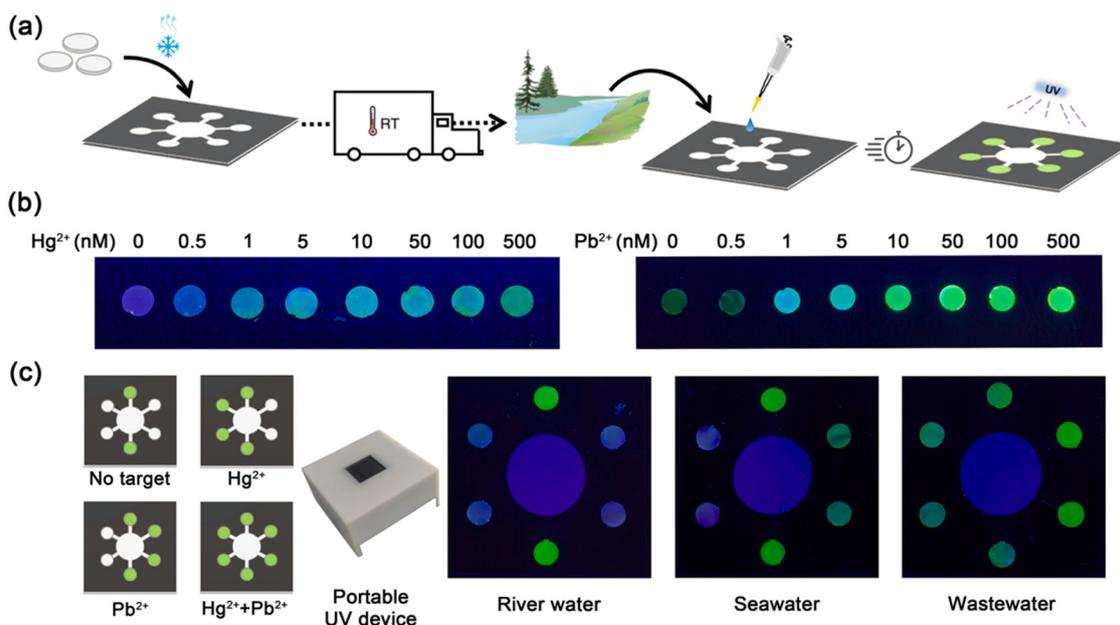
Fig. 9 (a) Schematic illustration of the development and application of paper-based biosensing device, (b) fluorescence output of paper-based biosensing device at different contents of Hg<sup>2+</sup> and Pb<sup>2+</sup>, and (c) detection of real water models using this inexpensive and portable paper-based biosensing device. Reproduced with permission from ref. 205 Copyright 2021, Elsevier.
