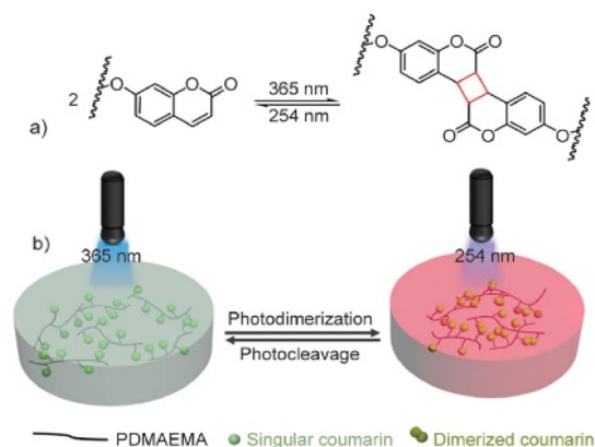
Fig. 55 (a) Reversible dimerization and cleavage of coumarin groups upon exposure to 365/254 nm light. (b) Schematic diagram of cross-linking network formation and dissociation. Reproduced from ref. 235 with permission from BME-PT, Copyright [2023].
