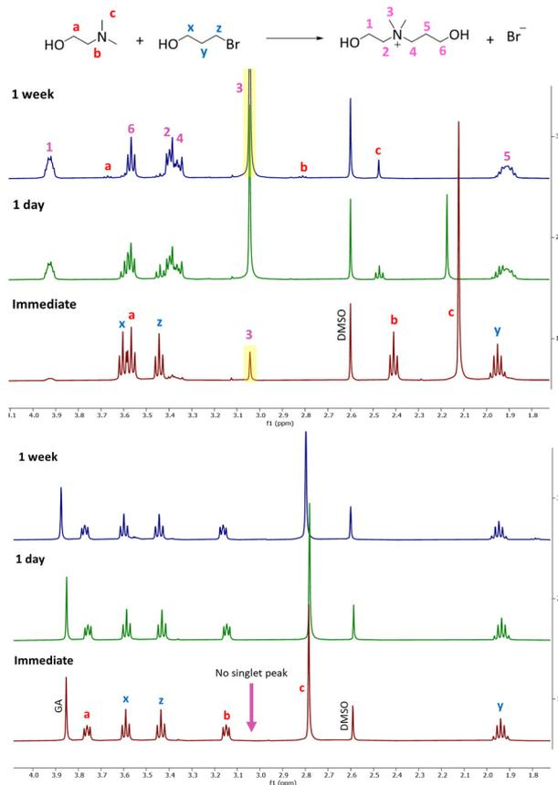
**Fig. 1** Overlaid <sup>1</sup>H NMR spectra of DMAE and BPO, when the amine is in the neutral state (above) and protonated state (below).
