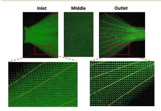
Fig. 2 Velocity vectors and streamlines at the inlet, middle section and outlet of the microfluidic chip for stimulated flow (13.125 mL h<sup>-1</sup>).
