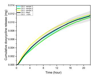
Fig. 4 Repeatability test in the microfluidic device. Three identical samples were tested, and the deviation of final drug concentration was less than 5%, pH 5.5, 37 °C cross sectional area of 7 mm², depth of 0.5 mm, and 10  $\mu$ L volume, unstimulated flow.
