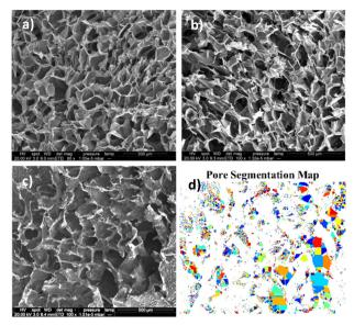
Fig. 6 SEM captured images of 3 (wt)% chitosan scaffold; a). 0 mg <sup>1</sup> doxycycline loaded, b). 10 mg ml<sup>-1</sup> doxycycline loaded, c). 40 mg ml<sup>-1</sup> doxycycline loaded; d) indicative segmentation map for determining porosity for 40 mg ml<sup>-1</sup> DOX sample.
