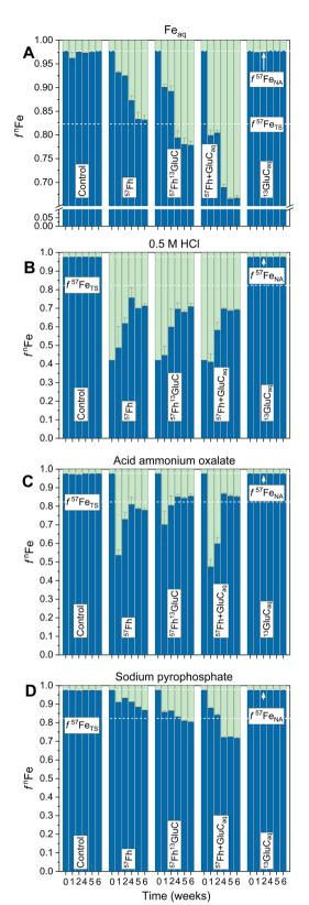
Fig. 1 Trends in Fe isotope composition of  $Fe_{aq}$  (A) and the selective chemical extractions, shown as f'Fe, where n=56 (blue) or 57 (green). (B) and (C) are steps 1 and 2 of the two-step sequential extraction whereby (B) is total Fe extracted with 0.5 M HCl (2 h) and (C) is Fe mobilized with an acid ammonium oxalate extraction. Panel (D) shows the isotope composition of Fe mobilized in the Na-pyrophosphate treatment. The initial timepoint (week 0) is calculated based on the
