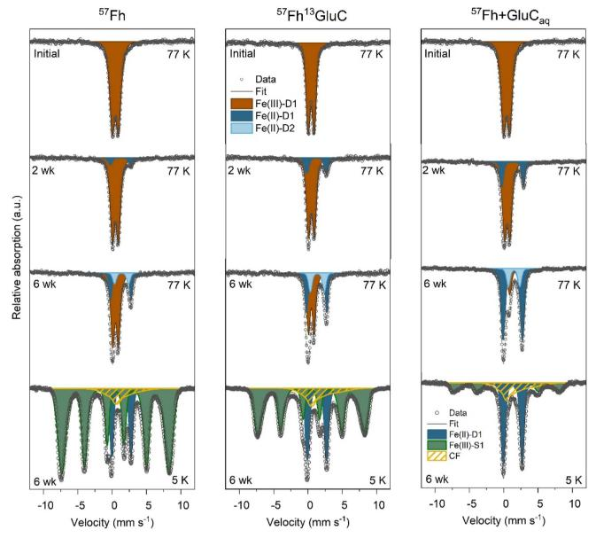
Fig. 3 77 K Mössbauer spectra of  $^{57}$ Fh,  $^{57}$ Fh + GluC<sub>aq</sub>, and  $^{57}$ Fh $^{13}$ GluC treatments prior to incubation (top row), after 2 weeks incubation (upper middle row), after 6 weeks incubation (lower middle row) and 5 K Mössbauer spectra of 6 weeks incubated samples (bottom row). Complete temperature profile spectra are shown in Fig. S10† and fit parameters are detailed in Table S9.†
