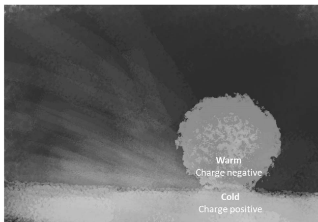
Fig. 2 Schematic representation of the effect of 'asymmetric rubbing' leading to electric charging of snow grains. Intensive friction creates higher temperature gradients and increases charge carrier concentration gradients because protons migrate faster toward cold regions.
