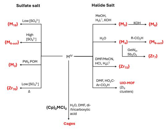
Fig. 19 Schematic diagram of the reaction path towards Zr/Hf clusters discussed in this article. The reaction path is applicable to both Zr(v) and Hf (v), (M = Zr, Hf), unless otherwise stated. L<sup>1</sup> can be either H<sub>3</sub>dihybo or H<sub>3</sub>pidiox, L<sup>2</sup> is 3,3',3'',3'''-(anthracene-9,10-diylidenebis(methane-1,1-diyl-1-ylidene))tetrabenzoic acid.
