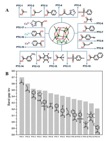
Fig. 10 O-donor ligands introduced in Ti<sub>6</sub> clusters (A). Band gap values of PTC-1 to PTC-14 (B). This figure has been adapted/reproduced from ref. 67 with permission from WILEY-VCH Verlag GmbH & Co, copyright 2016.
