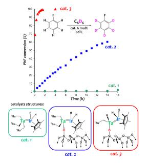
Fig. 6 Catalytic performances of Ta/Ir species in an arene hydrogen isotope exchange reaction between C<sub>6</sub>D<sub>6</sub> and fluorobenzene. 60,64
