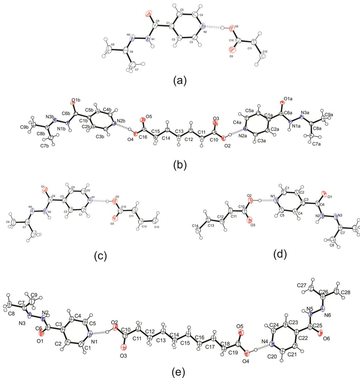
**Fig. 1** ORTEP diagram for the crystal structures presented in this work, (a) izact + C6, (b) izact + C7, (c) izact + C8, (d) izact + C9, and (e) izact + C10. Ellipsoids were calculated at 50% probability level.
