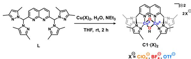
Scheme 1 Synthesis of **C1(X)<sub>2</sub>** complexes prepared in this work.
