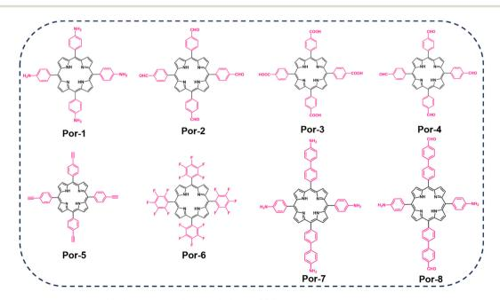
Fig. 2 Porphyrin monomers employed in the synthesis of porphyrin-based COFs.
