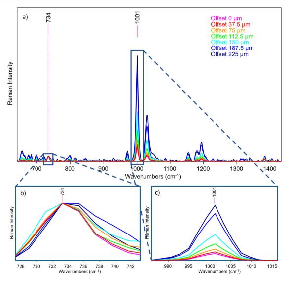
Fig. 6 (a) Portable fibre bundle micro-SORS measurement of S1; (b) all spectra have been normalized to the Teflon band (top layer) at 734 cm<sup>-1</sup>; (c) relative intensity increase of the polystyrene signal (bottom layer) (i.e. at 1001 cm<sup>-1</sup>) as the offset increases.
