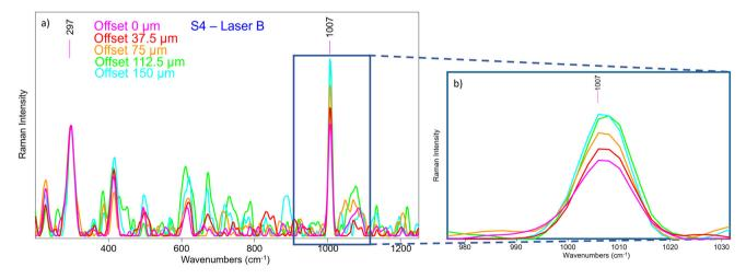
Fig. 12 (a) micro-SORS series acquired with the system coupled with Laser B in S4. All spectra have been normalized to the Sienna pigment characteristic band at 297 cm<sup>-1</sup>; (b) micro-SORS effect is visible through the increase of the gypsum (1007 cm<sup>-1</sup>) band of the preparation layer at the increasing of the offset.
