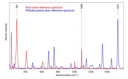
Fig. 7 Reference spectra of the two painted layers of S2, directly acquired on parts of the sample where they are not overlapped. The reference frequencies for each compound are indicated: 291 cm<sup>-1</sup> for red ochre, 1086 cm<sup>-1</sup> for calcite and 1531 cm<sup>-1</sup> for phthalocyanine blue.
