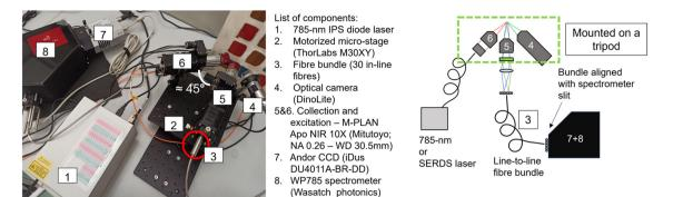
Fig. 2 Photo (a) and schematics (b) of the prototype with each component labelled.
