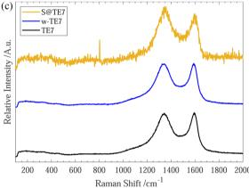
Fig. 2 (a) Raman spectra for SWCNT-121, w-SWCNT-121 and S@SWCNT-121, 532 nm excitation wavelength. (b) Raman spectra for SWCNT-777, w-SWCNT-777 and S@SWCNT-777, 532 nm excitation wavelength. (c) Raman spectra for TE7, w-TE7 and S@TE7, 532 nm excitation wavelength. All spectra are normalised to the intensity of the G-band for comparison. Each plot shows the as-purchased (black), washed (blue) and their sulfur composites (yellow).
