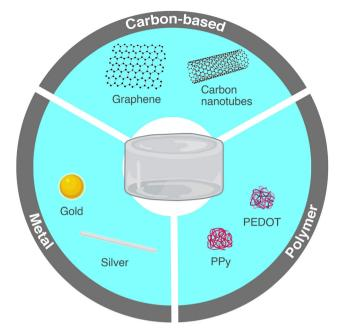
Fig. 6 Commonly used conductive nanomaterials in nanocomposite
