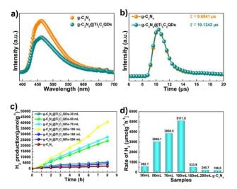
Fig. 8 (a) Steady photoluminescence (PL) and (b) time-resolved fluorescence decay spectra of  $g\text{-}C_3N_4$  and  $g\text{-}C_3N_4@\text{Ti}_3C_2$  QDs-100 mL composites,  $\lambda_{ex}=325$  nm. (c) Photocatalytic H $_2$  evolution and (d) rate of  $g\text{-}C_3N_4$  NSs, Pt/g-C $_3N_4$ , Ti $_3C_2$  MXene sheet/g-C $_3N_4$  and g-C $_3N_4@\text{Ti}_3C_2$  QDs. Reproduced with permission from ref. 123, Copyright 2019 The Royal Society of Chemistry.
