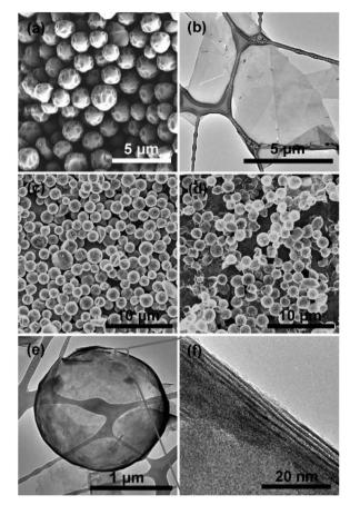
Fig. 5 (a) SEM images showing the morphology of the as-produced PMMA spheres. (b) TEM image of  $Ti_3C_2T_x$  flakes. SEM image of (c)  $Ti_3C_2T_x$ /PMMA hybrids and (d) hollow  $Ti_3C_2T_x$  spheres after removal of PMMA, showing that the spherical shape is retained after PMMA's thermal evaporation at 450 °C. TEM images showing (e) a hollow Ti<sub>3</sub>C<sub>2</sub>T<sub>x</sub> sphere and (f) its wall MXene layers. Reproduced with permission from ref. 84, Copyright 2017 Wiley Publications.
