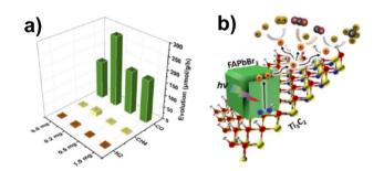
Fig. 11 (a) Photocatalytic CO<sub>2</sub> reduction performances of FAPbBr<sub>3</sub>/x-Ti<sub>3</sub>C<sub>2</sub> (x = 0.0, 0.2, 0.5, and 1.0) in deionized water under AM 1.5 G (150 mW cm<sup>-2</sup>). (b) Schottky heterojunction photocatalytic system for CO<sub>2</sub> reduction in FAPbBr<sub>3</sub>/x-Ti<sub>3</sub>C<sub>2</sub>. Reproduced with permission from ref. 146, Copyright 2021 American Chemical Society.
