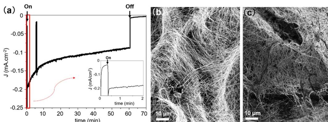
Fig. 7 (a) Chronoamperometry of PCS-SiNW-MoS<sub>x</sub> at -0.15 V vs. RHE in 0.5 M H<sub>2</sub>SO<sub>4</sub> under illumination (48 nm-SiNWs, Δ*Q*<sub>MoS<sub>x</sub></sub> = 6 mC cm<sup>-2</sup>) with N<sub>2</sub> bubbling. SEM images of the electrode before (b) and after (c) the stability test.
