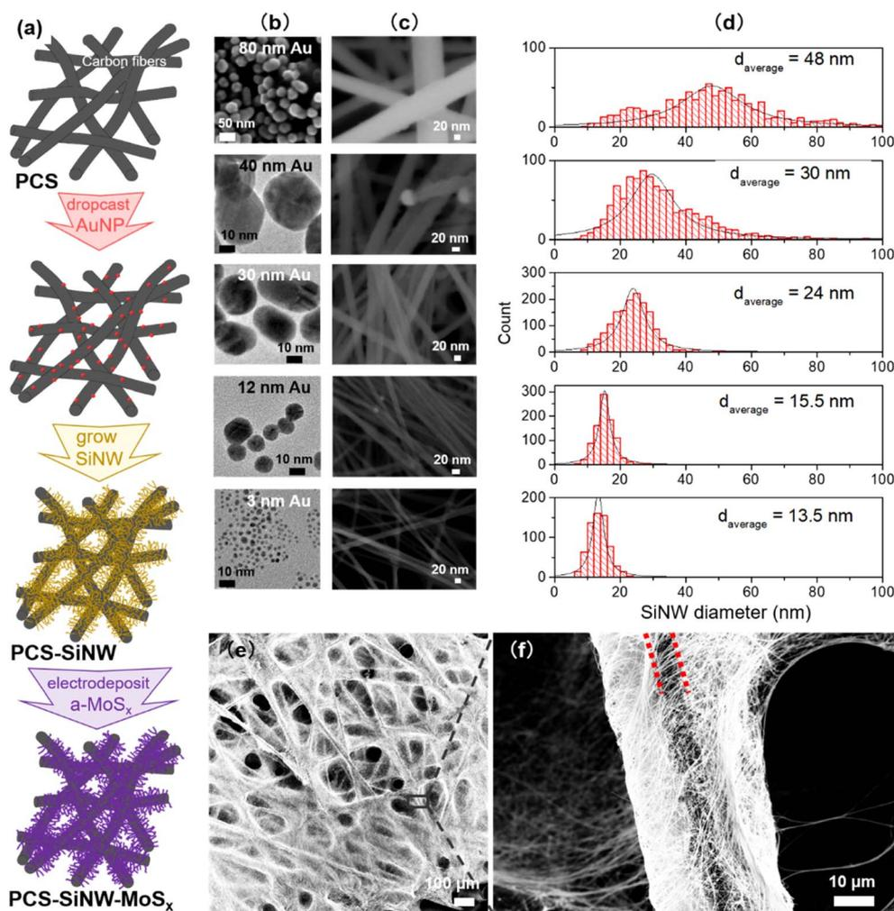
Fig. 2 Tuning SiNW diameter by the size of AuNPs: (a) scheme of the PCS-SiNW-MoS<sub>x</sub> photocathode fabrication. SEM and TEM images of the AuNPs of size 3–80 nm (b) and the subsequent SiNWs grown from them (c); (d) corresponding SiNW diameter histograms (>500 counts); SEM images of the PCS-SiNW (e) and close up view of a single carbon fiber (f). Red dotted lines highlight the diameter of the carbon fiber.
