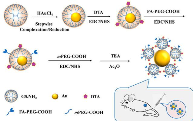
Fig. 6 Schematic presentation of the preparation of Au DSNs–DTA–FA for targeted enhanced CT imaging of tumors. Reproduced with permission.<sup>17</sup> Copyright 2020, American Chemical Society.
