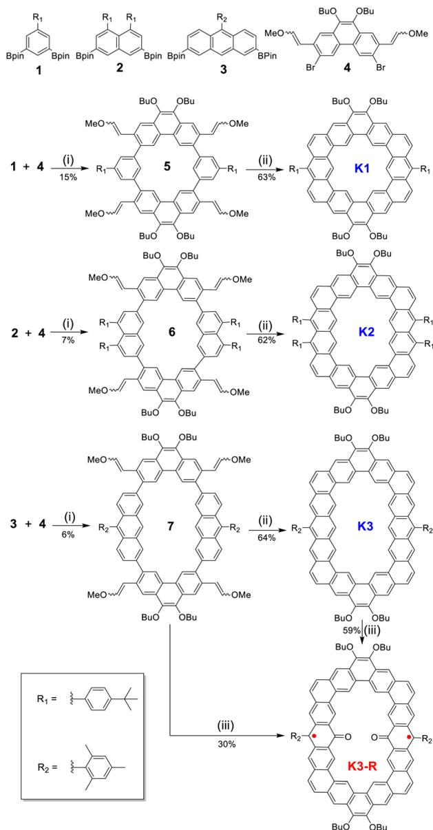
Scheme 1 Synthetic route of alkoxy- and aryl-cosubstituted cycloarenes **K1**–**K3** and carbonylated cycloarene diradical **K3-R**: (i) XPhos Pd G2, K<sub>3</sub>PO<sub>4</sub>, THF/H<sub>2</sub>O, 50 °C; (ii) Bi(OTf)<sub>3</sub>, CH<sub>2</sub>ClCH<sub>2</sub>Cl, rt; (iii) Bi(OTf)<sub>3</sub>, air (O<sub>2</sub>), CH<sub>2</sub>ClCH<sub>2</sub>Cl, 80 °C.
