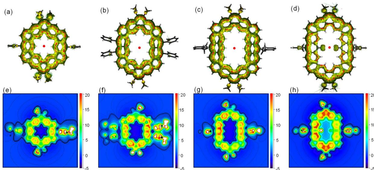
Fig. 4 Calculated ACID plots (contribution from π-electrons only) of (a) **K1**, (b) **K2**, (c) **K3**, and (d) **K3-R**. The magnetic field is perpendicular to the XY plane and points out through the paper. The red arrows indicate the clockwise (diamagnetic) current flow. Calculated 2D ICSS<sub>zz</sub> maps for (e) **K1**, (f) **K2**, (g) **K3**, and (h) **K3-R**.
