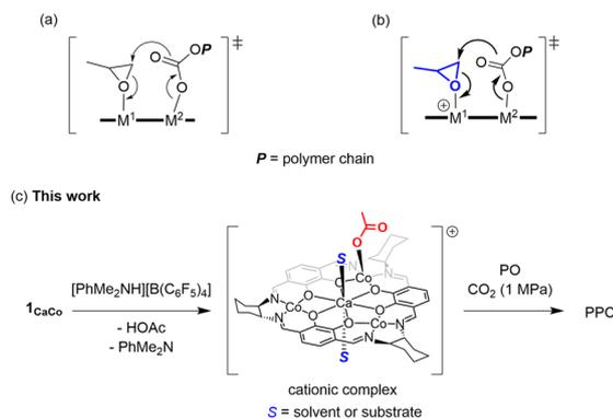
Scheme 1 Key transition state structures of (a) neutral multinuclear catalysts, (b) cationic multinuclear catalysts. (c) This work: alternating copolymerization of PO and CO<sub>2</sub> by cationic multinuclear species in the presence of anilinium salt.
