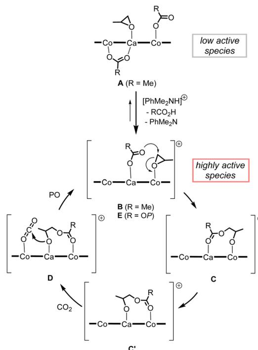
Scheme 4 Plausible reaction mechanism of alternating copolymerization of PO and CO<sub>2</sub> mediated by complex **1**<sub>CaCo</sub> with anilinium borate.
