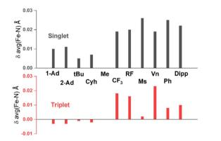
Fig. 6 Imido-substituent-dependent deviation of average Fenk(imido) distance relative to that of the methyl substituent obtained from DFT optimization. The substituents on NHC side are two methyl groups in all cases presented here. Full data can be found in Table S2.† Abbreviations: Ad = adamantyl, tBu = tert-butyl, Cyh = cyclohexyl,  $RF = C(CF_3)_3$ ,  $CF = C(CF_3)$
